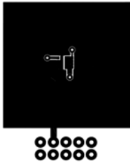
a. 65^\circ\text{C/W} when mounted on a 1\text{ in}^2 pad of 2 oz copper
