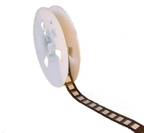
Figure 17: Reeled SARA-U2 modules
