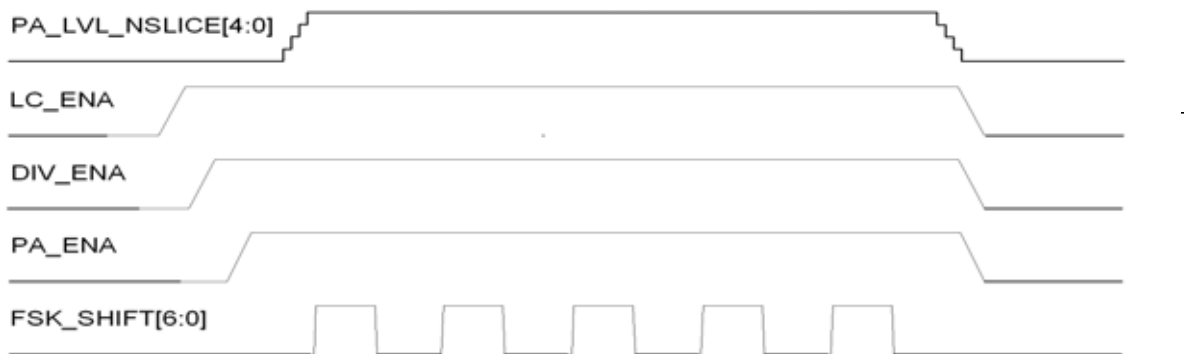
Figure 13.2. FSK Timing Example
