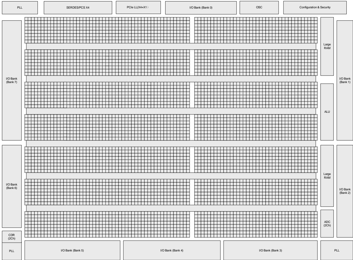
Figure 2.1. Simplified Block Diagram, LFCPNX-50 Device (Top Level)
