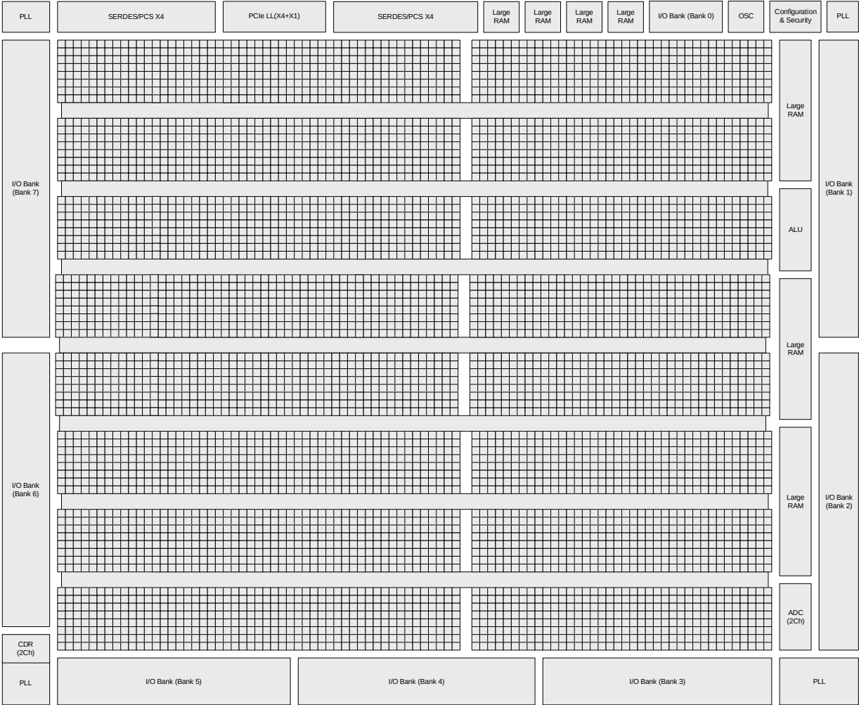
Figure 2.2. Simplified Block Diagram, LFCPNX-100 Device (Top Level)
