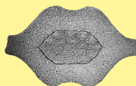
H shape cross section turned contact
