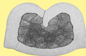
B shape cross section stamped contact
