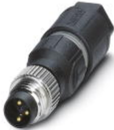
Sensor/actuator connector, male connector, straight, 3-pos., M8, QUICKON-ONE, metal knurl, maximum cable diameter of 5.0 mm
