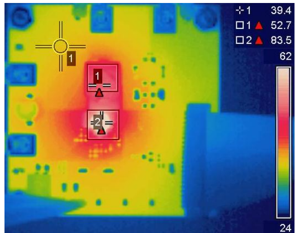
Figure 19: Thermal Image at V_{IN} = 16V , I_{OUT} = 10A (IR3865: 84°C, Inductor: 53°C, PCB: 39°C)
