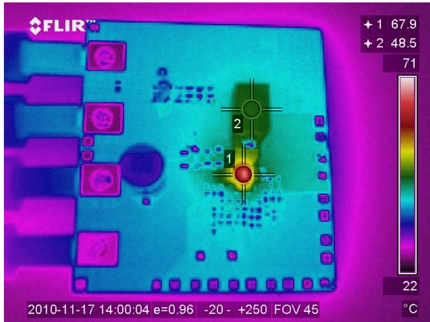
Figure 40: Thermal Image of the Board at 9A Load, Test Point 1 is IR3899, Test Point 2 is inductor
