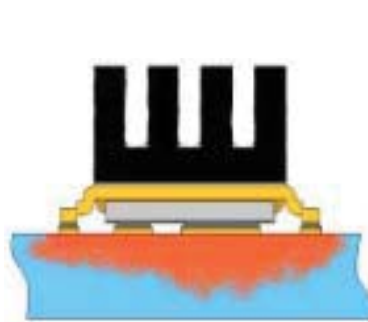
④ Mounted to a PCB with small clip heatsink (still air)
