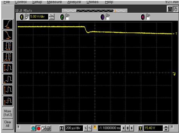
FIGURE 10. VLNB TRANSITIONS FROM 18.3V TO 13.3V
