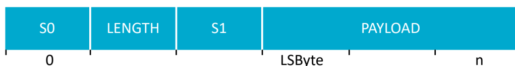
Figure 111: Representation of a RADIO packet in RAM
