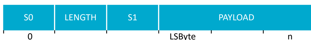
Figure 111: Representation of a RADIO packet in RAM
