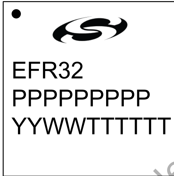
Figure 8.3. QFN32 Package Marking
