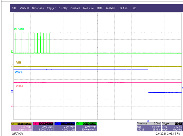
Figure 9-10. Shipmode Entry on VIN Removal
