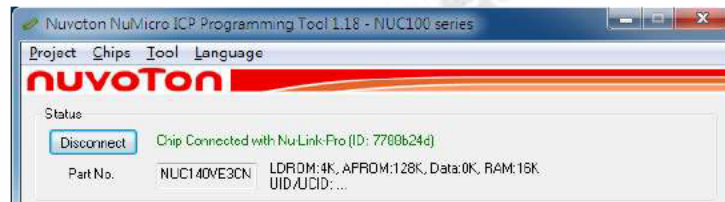
Figure 4-7 Nu-Link Adapter Connected with a Target Chip Detected
