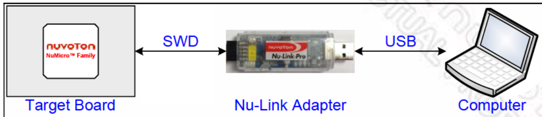
Figure 4-1 Nu-Link Adapter Connection Diagram
