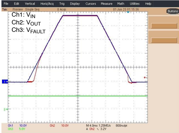
Figure 14. Turning on a Single Output with the Input Voltage (EN pin pull-up or floated)
