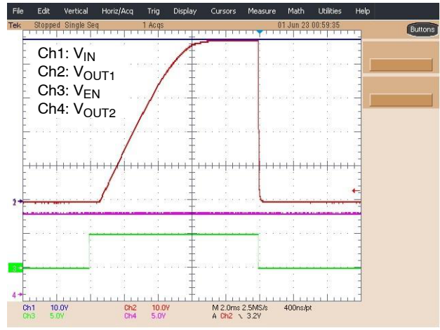
Figure 13. Turning on a Single Output with the EN Pin While Another Output Pin is On
