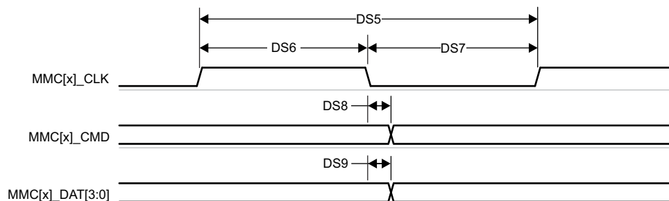
Figure 7-92. MMCSD1 – Default Speed – Transmit Mode
