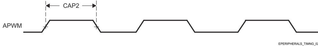
Figure 7-51. ECAP Output Timings
