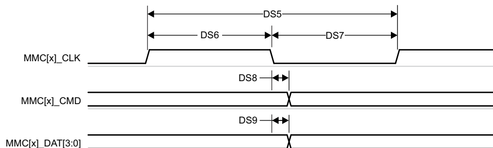
Figure 7-92. MMCSD1 – Default Speed – Transmit Mode
