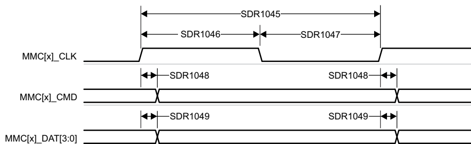
Figure 7-101. MMCSD1 – UHS-I SDR104 – Transmit Mode
