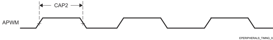
Figure 7-51. ECAP Output Timings
