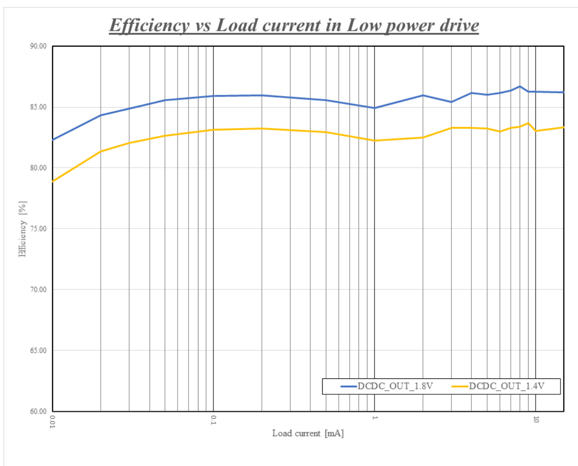
Figure 5. Efficiency vs Load current in Low-power drive
