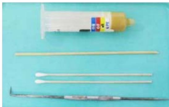
Figure 10-5: Underfill Rework Tools
