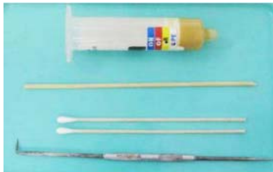
Figure 10-5: Underfill Rework Tools
