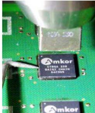
Figure 10-7: Removing Underfill Using Steel Probe
