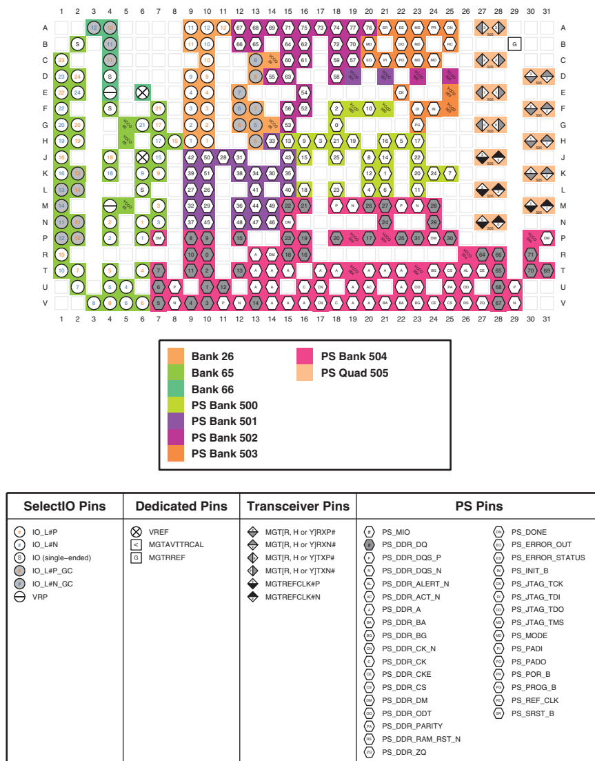
Figure 4-7: UBVA530 Package—XCZU2CG, XCZU2EG, XCZU3CG, and XCZU3EG I/O Bank Diagram
