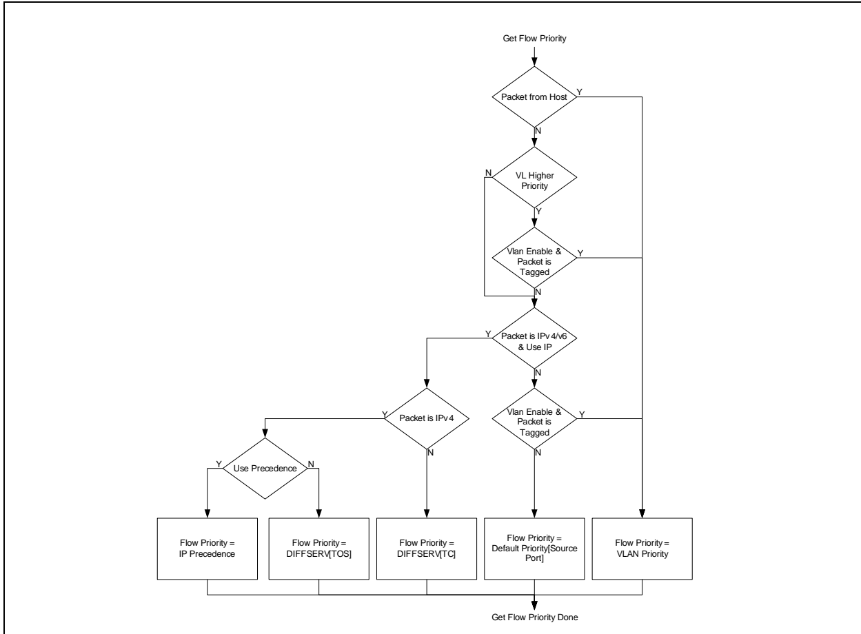
FIGURE 6-7: SWITCH ENGINE INGRESS FLOW PRIORITY CALCULATION
