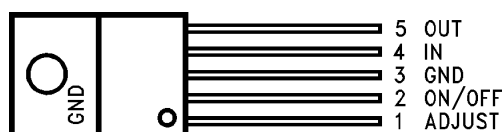
Figure 8. TO-220 5-Lead Power Package Front View
