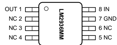
LM2936MM VSSOP (DGK) Package 8-Pins Top View
