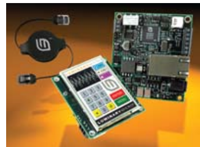
Stellaris Intelligent Display Module Reference Design Kit
