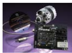
Stellaris AC Induction Motor Reference Design Kit
