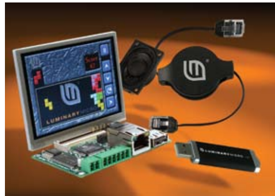
Stellaris Intelligent Display Module Single-Board Computer
