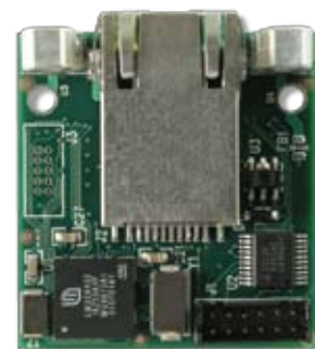
Stellaris Serial-to-Ethernet Module
