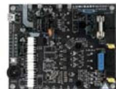
Stellaris AC Induction Motor Module
