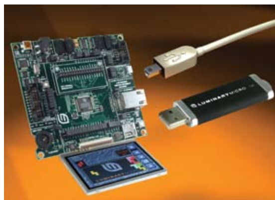
Stellaris LM3S9B96 Microcontroller Development Kit
