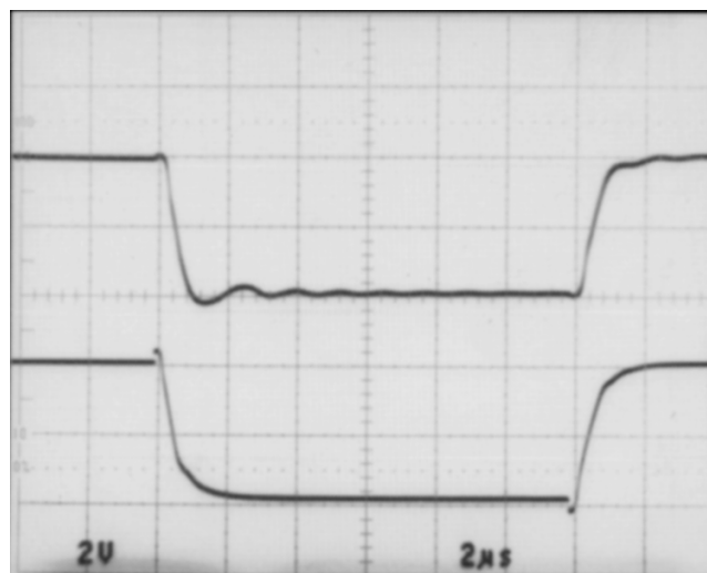
Figure 32. Four-Volt Step Response: with Cap Load (Top Trace) without Cap Load (Bottom Trace)
