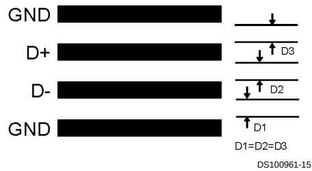
FIGURE 6. Recommended Diode Trace Layout
