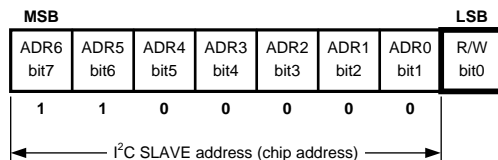
Figure 41. I 2 C Chip Address (see note above)
