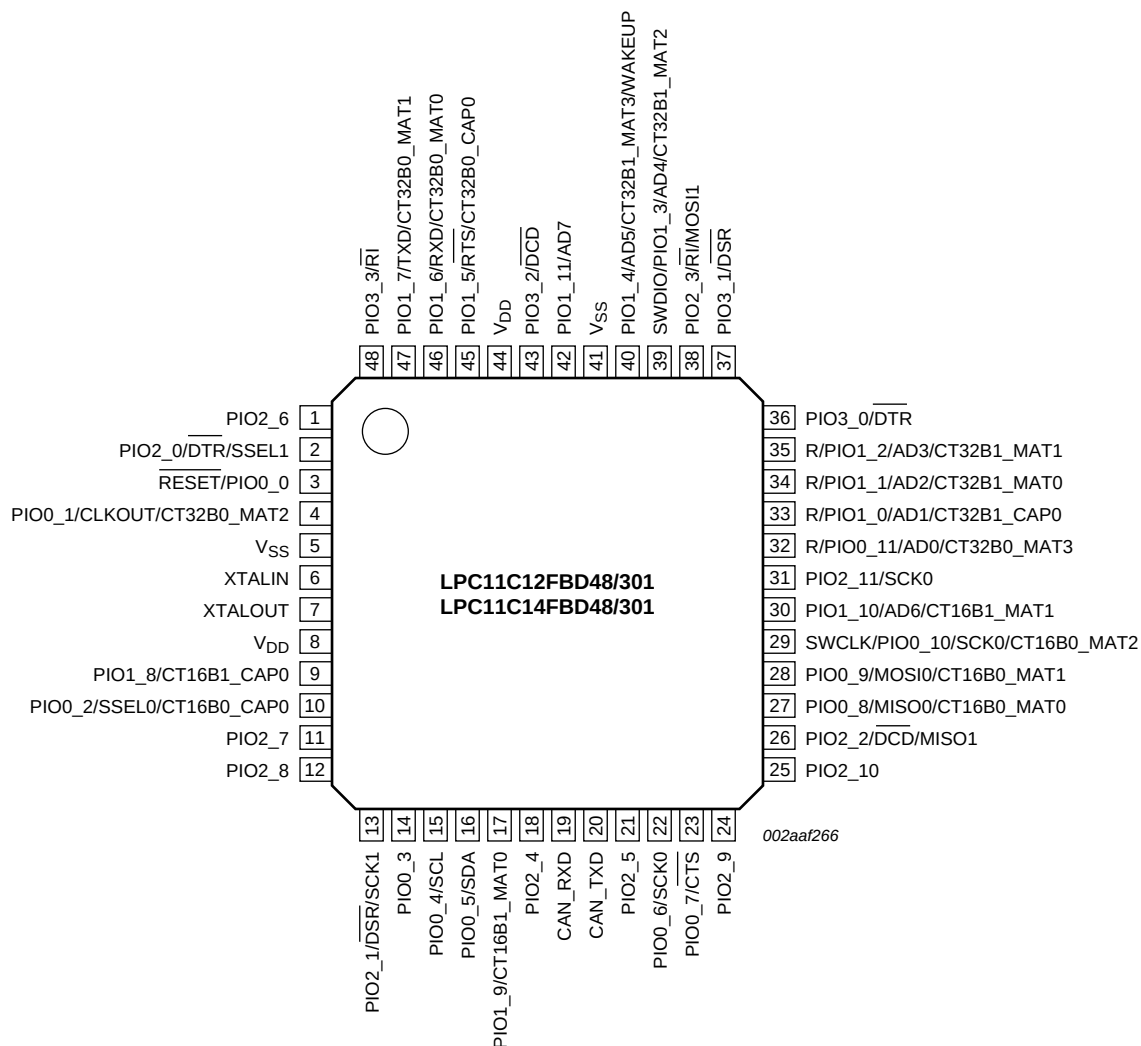
Fig 19. Pin configuration LQFP48 package
