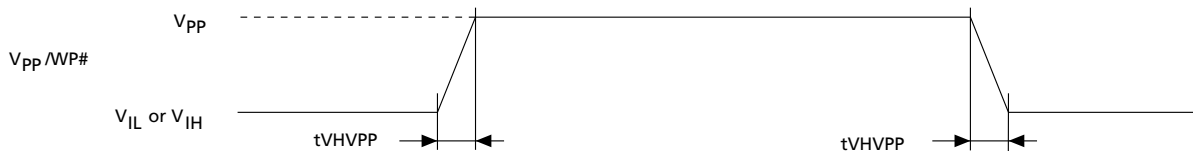
Figure 24: Accelerated Programming Timing Waveform
