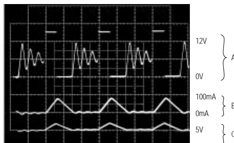
MAX758A SWITCHING WAVEFORMS DISCONTINUOUS CONDUCTION
