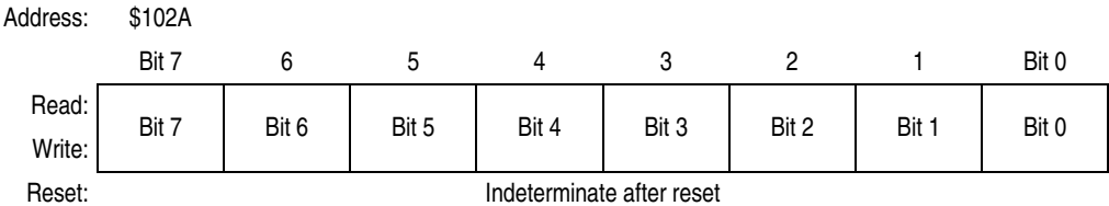
Figure 8-5. Serial Peripheral Data I/O Register (SPDR)
