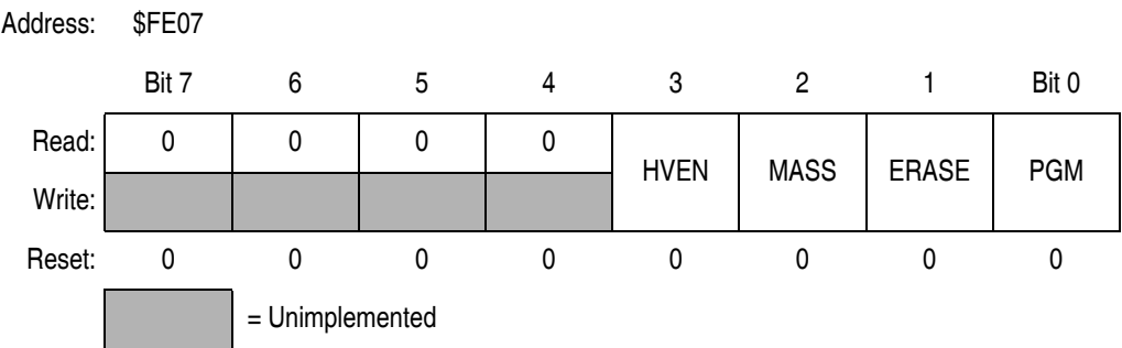
Figure 4-1. FLASH Control Register (FLCR)
