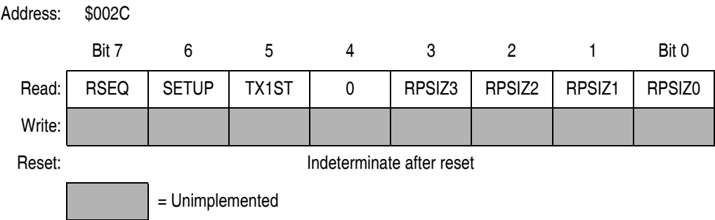
Figure 13-7. USB Status Register (USR)
