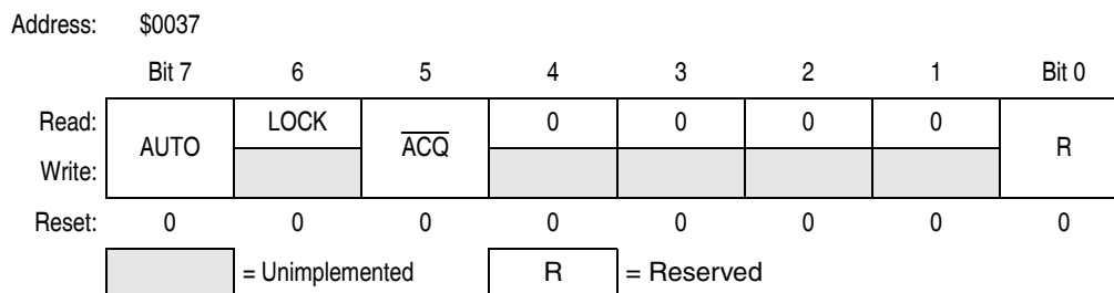
Figure 4-5. PLL Bandwidth Control Register (PBWC)
