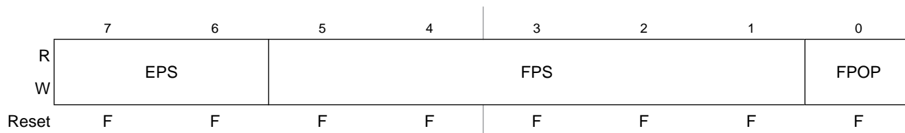
Figure 4-17. FLASH and EEPROM Protection Register (FPROT)
