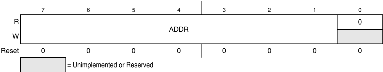
Figure 13-3. IIC Address Register (IIC1A)
