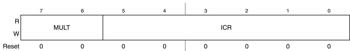
Figure 13-4. IIC Frequency Divider Register (IIC1F)
