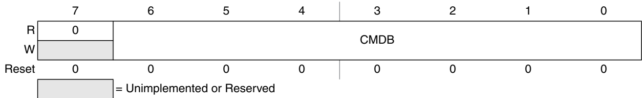
Figure 2-11. Flash Command Register (FCMD - NVM User Mode)
