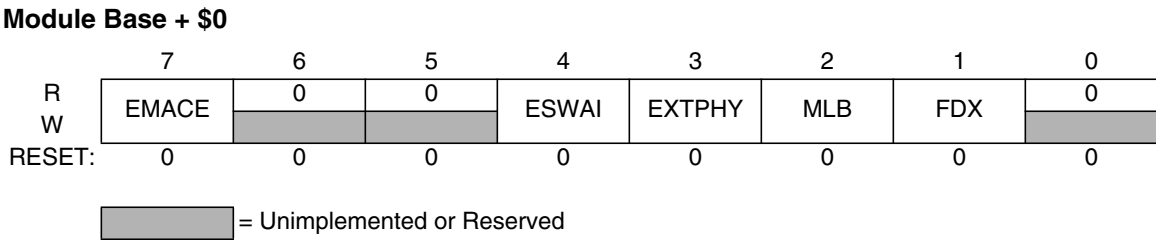
Figure 11-2. Network Control (NETCTL)
