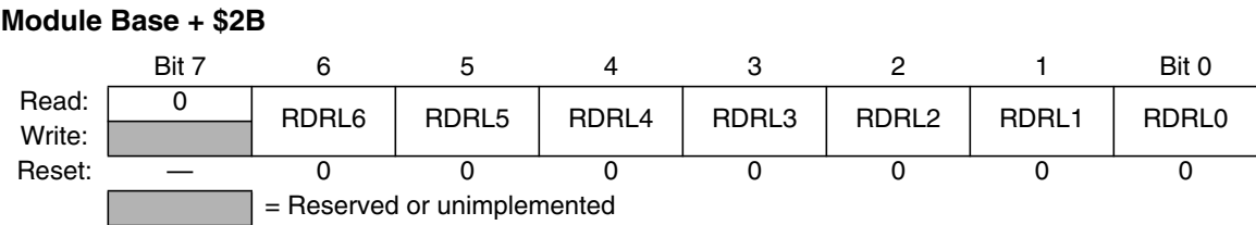
Figure 3-42. Port L Reduced Drive Register (RDRL)
