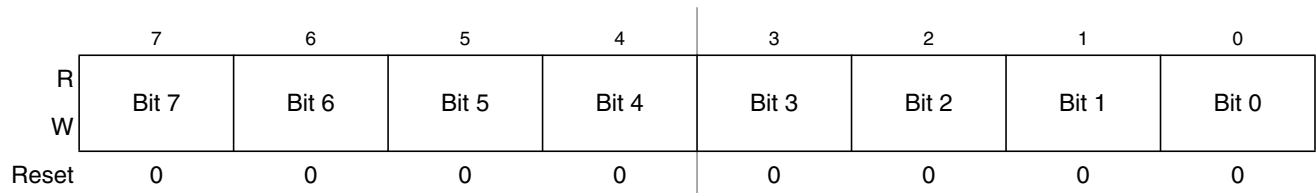
Figure 18-18. Debug Comparator A Register Low (DBGCAL)
