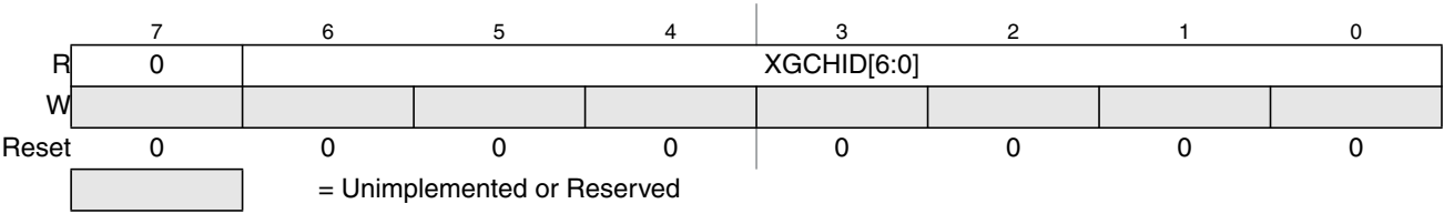
Figure 10-4. XGATE Channel ID Register (XGCHID)
