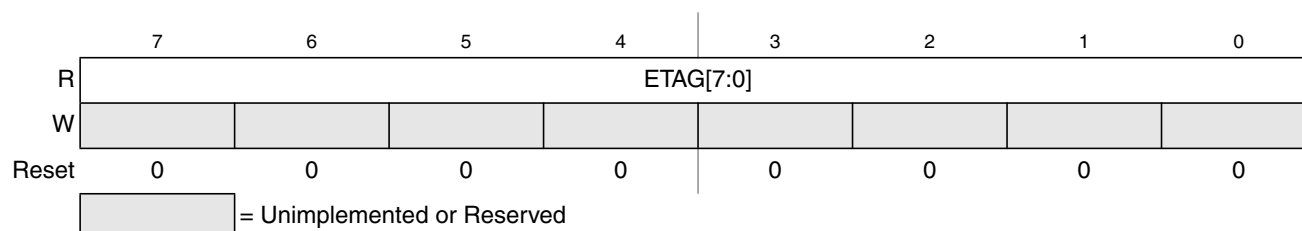
Figure 25-19. EEE Tag Counter Low Register (ETAGLO)
