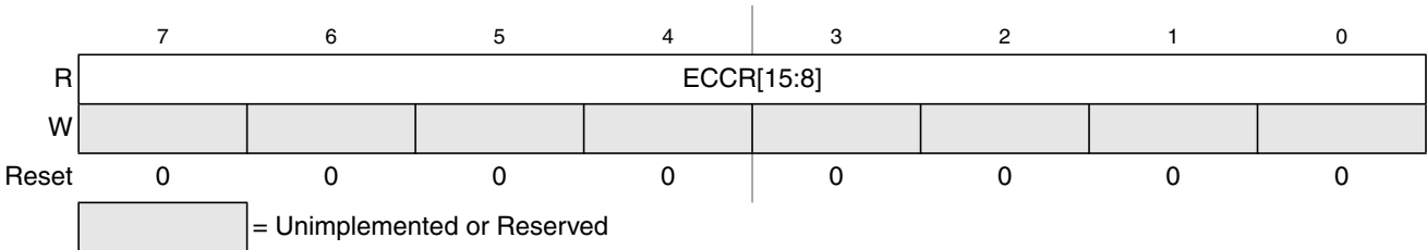
Figure 26-20. Flash ECC Error Results High Register (FECCRHI)
