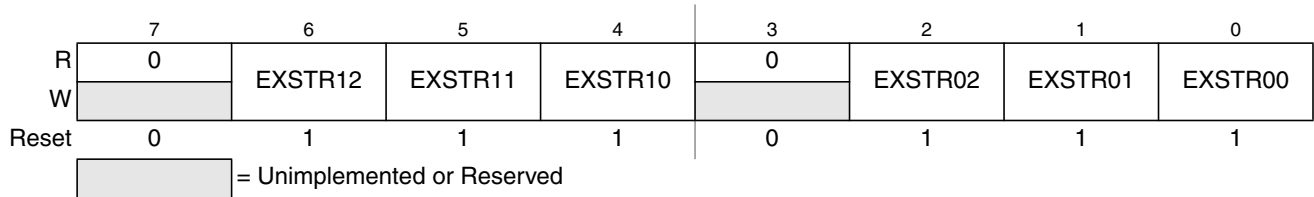
Figure 5-4. External Bus Interface Control Register 1 (EBICTL1)
