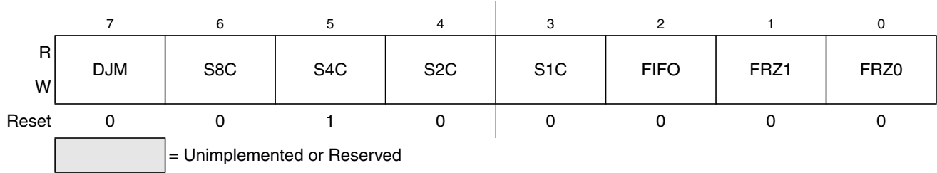
Figure 13-6. ATD Control Register 3 (ATDCTL3)
