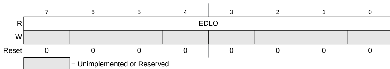
Figure 4-16. EEPROM Data Low Register (EDATALO)
