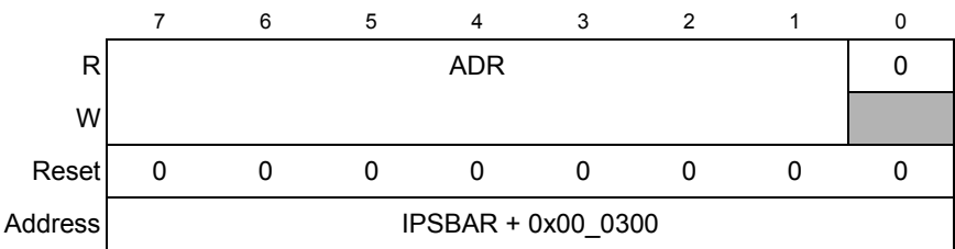
Figure 25-9. I 2 C Address Register (I2ADR)
