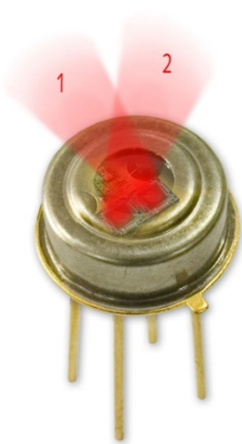
Figure 31: Identification of zone 1&2 relative to alignment tab
